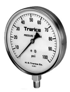
These rugged gauges with stainless steel case are big enough to read accurately for service or test purposes. The break-resistant plastic lens will survive the service truck. Lower cost "tin can" gauges have their purpose but are usually lower accuracy, averaging 2–3% of full scale. Compound ranges are useful for reading pump pressures which sometimes pull a vacuum on startup and can damage the pointer. Gauges shown are 1/4″ bottom mount. Slotted zero adjustment on the dial face.
