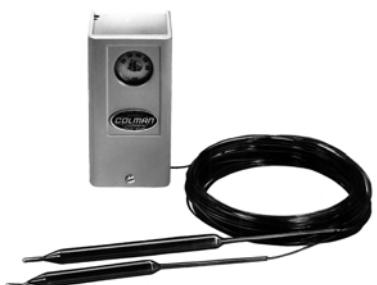
This control provides a simple method of changing the controlled setpoint in relation to the outdoor temperature. One bulb senses the controlled media, the second bulb senses the outdoor air temperature. The temperature of the controlled media increases as the outdoor air temperature decreases, thus providing only the minimum heat necessary for the ambient conditions. This results in decreased heat loss and results in considerable energy savings.
