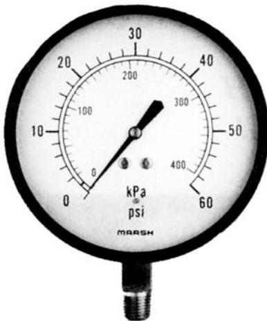
These gauges have a front bezel and a rear clamp to mount in panel doors. They are inserted into the hole in the front and clamped in the rear for a clean panel look. Models shown have 1/4" MPT back connection. Other ranges up to 5000 psi are also available in back and bottom mount. Smaller sizes are also available in 1/8" back mount.
