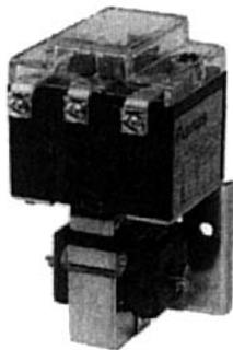
The alternator relay provides a means of automatically alternating the operation of two separately mounted motor driven pumps or compressors. Each time a pressure increase is required by the system, the alternating action assures even readiness and wear on both pumps.
