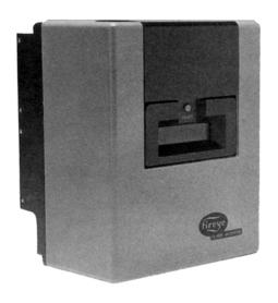
The Fireye Flame Monitor System is a microprocessor-based burner management control system with self-diagnostics, non-volatile memory and a vocabulary of 42 different messages. The monitor's message center provides the operator with scroll-out information.
