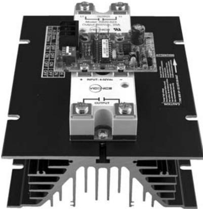
SCR power controllers are designed for an accurate and cost effective way to modulate electric heat. Useful for electric reheat and supplemental electric duct heaters. Viconics' R820 SCR power controller has been designed for safe and reliable control of electric heat loads. As a result, this broad line of products is used by most major North American duct heater manufacturers.
