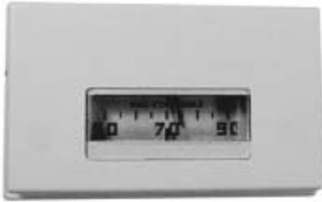
The KMC STE-5200/5300 series room temperature sensors are designed for use in KMC Digital or other building automation systems. They incorporate a 10,000 W (@ 77°F) thermistor for the sensing element, providing precise, stable temperature sensing. All models provide 10,000 W (5,000 W @ 70°F) setpoint adjustment capability which may be restricted to a single setpoint or specific range.
