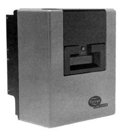
The **Fireye Flame Monitor System** is a microprocessor-based burner management control system with self-diagnostics, non-volatile memory and a vocabulary of 42 different messages. The monitor's message center provides the operator with scroll-out information.
