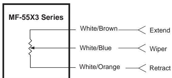
Figure-2 15K Feedback Potentiometer for MF-55X3 Series Models.
