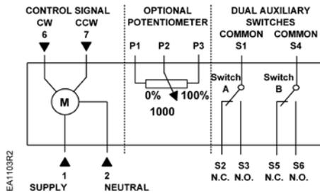
Figure 25. GCA13x, Floating Control.
