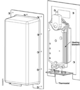
**Figure 11. Heater/Weather Shield Assembly.**
