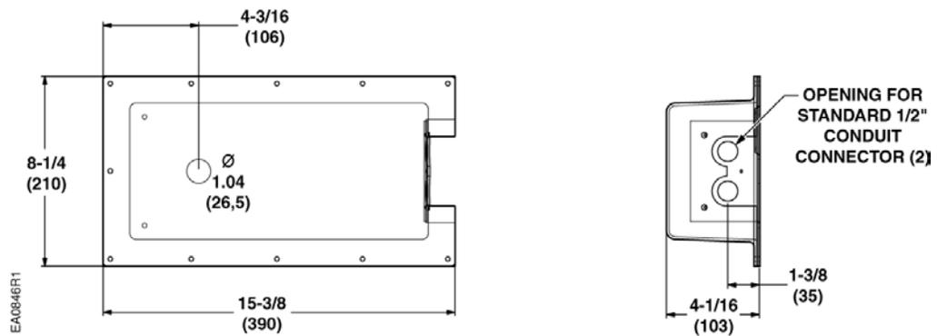
Figure 29. Dimensions of the ASK75.1U Weather Shield in Inches (Millimeters).
