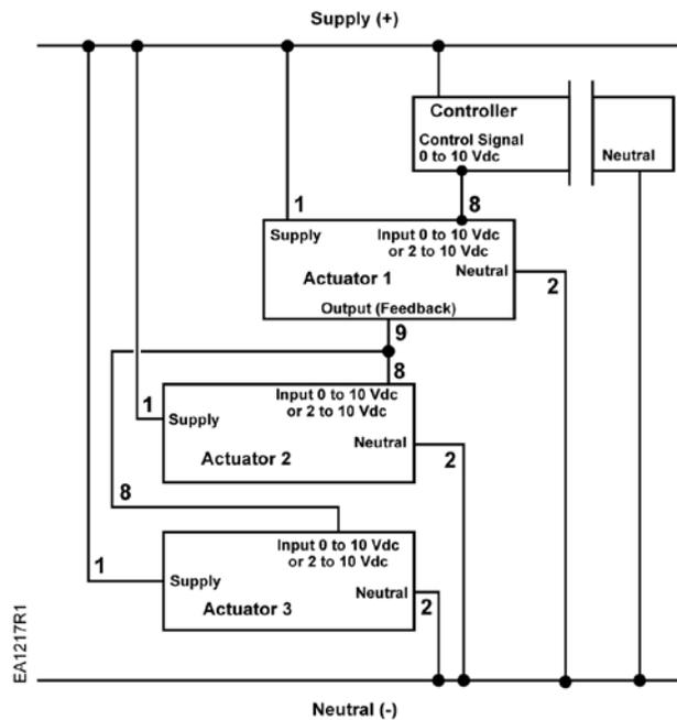
Figure 27. GCA15x.1x for Tandem Application (Master/Slave).
