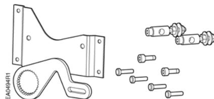
**Figure 5. Crank Arm Kit with Mounting Bracket.**
