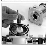
Remove thermal housing cap screws and lift out thermal element.
