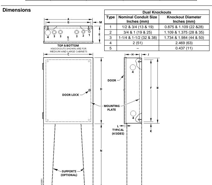
Figure 4. Cabinet and Support Dimensions (See Table 5 and Figure 9).
