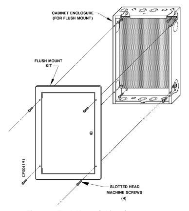
Figure 3. Flush Mount Cabinet Components.
