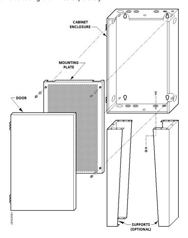
Figure 2. Wall Mount Cabinet Components.
