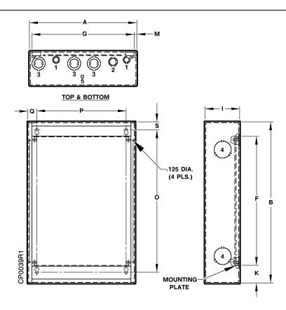
Figure 7. Flush Mount Cabinet Dimensions (See Table 7).
