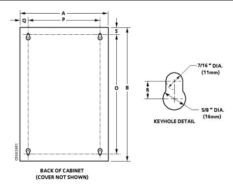
Figure 5. Rear View of Cabinet (See Table 6).
