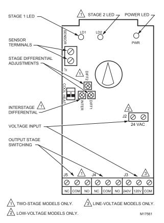
Fig. 5. Board layout for T7079.
