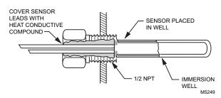
Fig. 3. Sensor inserted in an immersion well.
