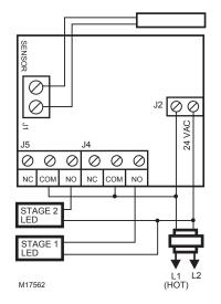
Fig. 6. Typical low-voltage (24 Vac) wiring application.
