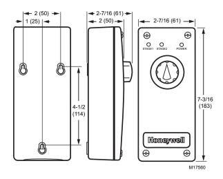
Fig. 1. Dimensions of T7079 in in. (mm).
