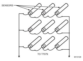
Fig. 2. Parallel-series wiring of sensors.
