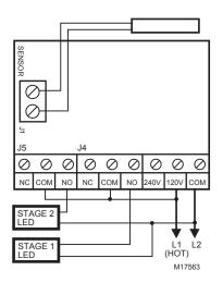
Fig. 7. Typical line-voltage (120 Vac) wiring application.
