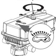
When handcrank is connected to actuator, the motor & signal control will be disabled
