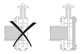
Is it possible for a butterfly valve to be installed in the line without an actuator?
