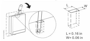
2. If needed, disconnect the cables or detach the rear module by unscrewing the screws anticlockwise. Or, if there is decoration frame, detach it as well by unscrewing the screws.
