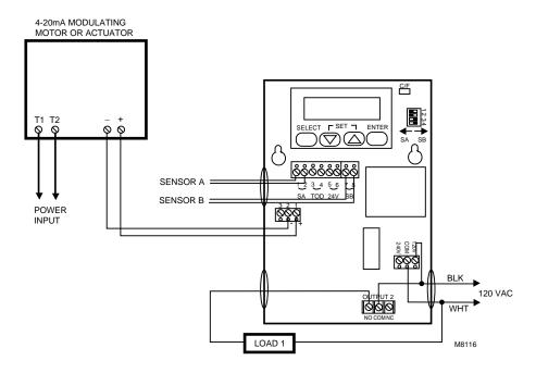
Fig. 12. Reset control with 120 Vac input, 4 to 20 mA and 120 Vac loads.
