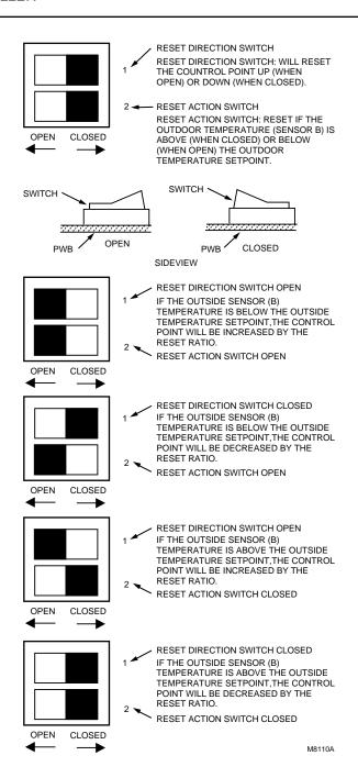
Fig. 18. Reset switch configuration.
