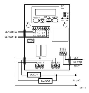
Fig. 10. Reset control with 120 Vac input, 24 Vac loads.
