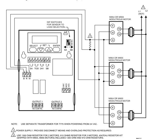
Fig. 14. Reset control with Series 90 Modutrol® Motor.
