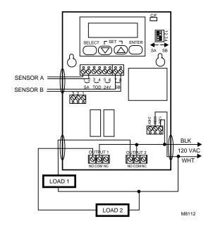
Fig 8. Reset control with 120 Vac input, 120 Vac loads.
