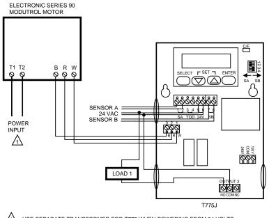
USE SEPARATE TRANSFORMER FOR T775 WHEN POWERING FROM 24 VOLTS.
