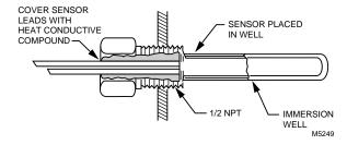
Fig. 4. Sensor inserted in immersion well.
