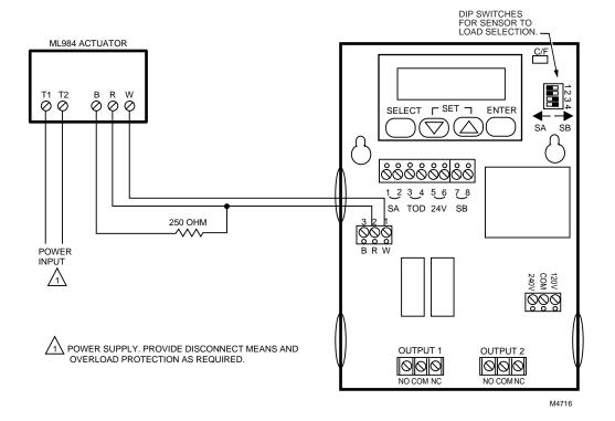
Fig. 15. Reset control with ML984 Valve Actuator.
