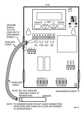
Fig. 6. Using shielded cable for cable runs longer than 25 feet.
