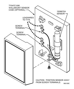
Fig. 3. Sensor mounted on wall.
