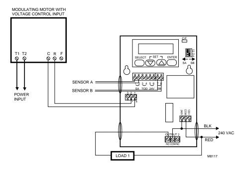
Fig. 13. Reset control with 240 Vac input, 240 Vac and 0 to 18 Vdc loads.
