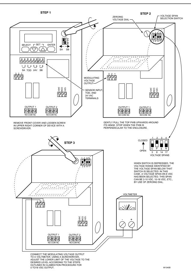
Fig. 16. Voltage span selection.
