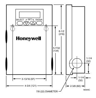
Fig. 1. Approximate T775J dimensions in in. (mm).
