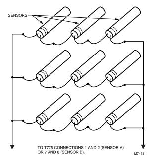
Fig. 2. Parallel-series wiring of sensors.
