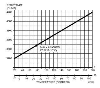
Fig. 21. Resistance versus temperature performance characteristics.
