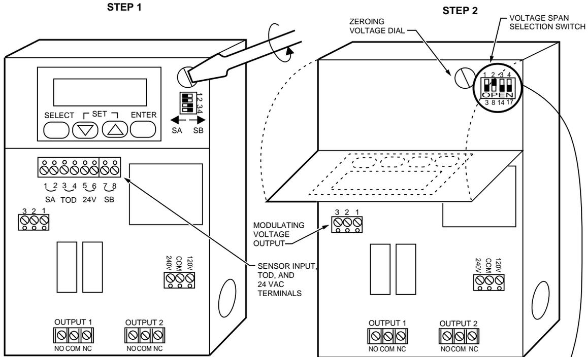
REMOVE FRONT COVER AND LOOSEN SCREW IN UPPER RIGHT CORNER OF DEVICE WITH A SCREWDRIVER.
