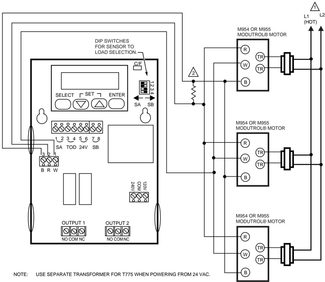
NOTE: USE SEPARATE TRANSFORMER FOR T775 WHEN POWERING FROM 24 VAC.
