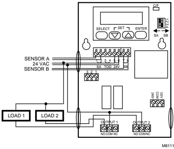
Fig. 7. Reset control with 24 Vac input, 24 Vac loads.
