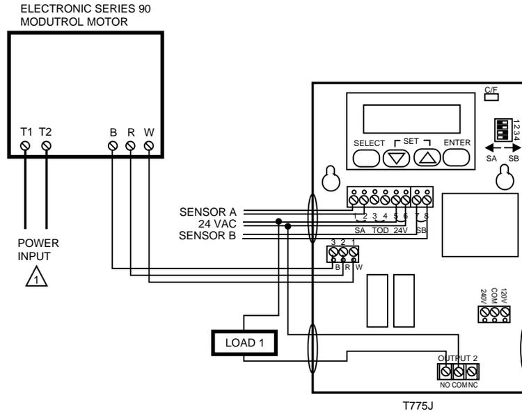
1 USE SEPARATE TRANSFORMER FOR T775 WHEN POWERING FROM 24 VOLTS.
