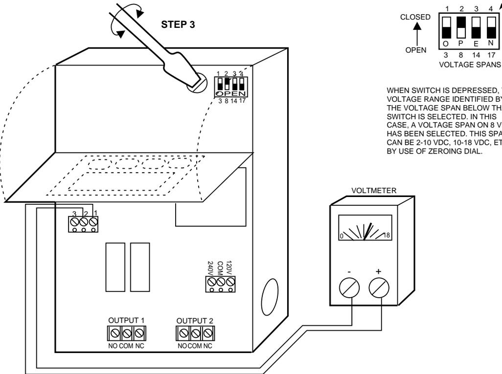
CONNECT THE MODULATING VOLTAGE OUTPUT TO A VOLTMETER. USING A SCREWDRIVER, ADJUST THE LOWER LIMIT OF THE VOLTAGE TO THE DESIRED LEVEL ACCORDING TO THE STEPS OUTLINED IN CLAIBRATION PROCEDURE FOR 0 TO18 VDC OUTPUT.
