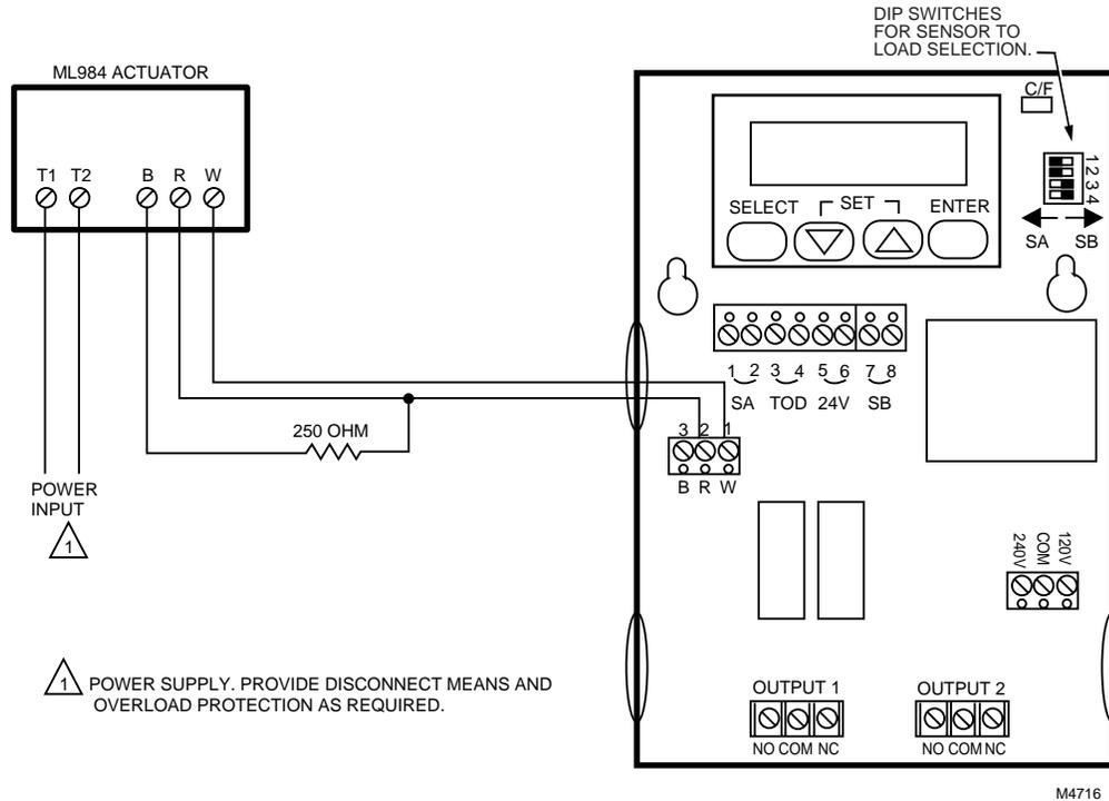
Fig. 15. Reset control with ML984 Valve Actuator.
