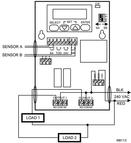
Fig. 9. Reset control with 240 Vac input, 240 Vac loads.
