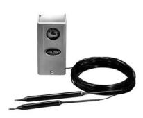
This control provides a simple method of changing the controlled setpoint in relation to the outdoor temperature. One bulb senses the controlled media, the second bulb senses the outdoor air temperature. The temperature of the controlled media increases as the outdoor air temperature decreases, thus providing only the minimum heat necessary for the ambient conditions. this results in decreased heat loss and results in considerable energy savings.
